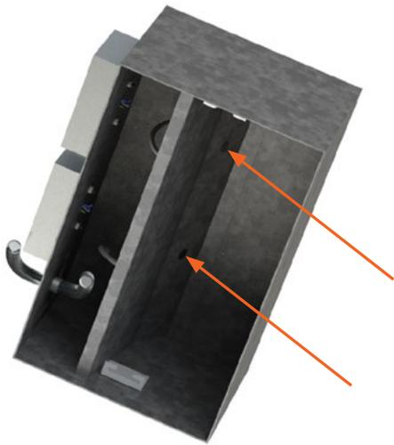
2. Unscrew electrical panel to access wiring. Cut electrical connections from ballasts and power and remove any loose wiring.
